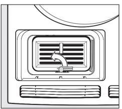
Turn the lever on the condenser unit upwards to the vertical position.
